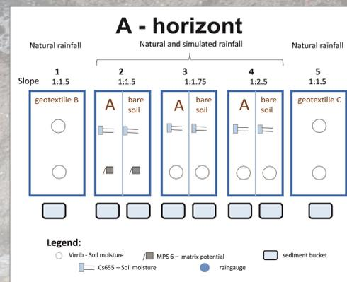
Figure 3 Experimental plots at the field rainfall simulator.
