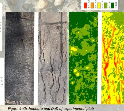
Figure 9 Orthophoto and DoD of experimental plots.
