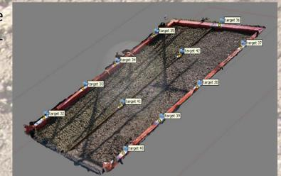
Figure 2 Experimental plot divided on 2 halves - left one covered with tested geotextile and right one with bare soil without any protection.
