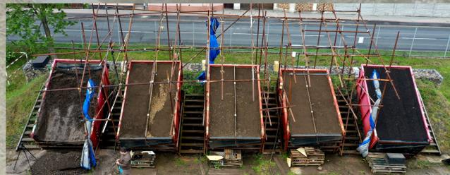
Figure 1 Field rainfall simulator and experimental plots for testing rolled erosion control products (RECPs)
